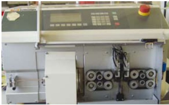
Automatic cutting and stripping
